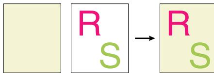
FIGURE 13.4 In the DjVu rendering model, objects are rendered, with their assigned colors, onto a background plane. There is neither explicit mask plane nor FG bitmaps.
